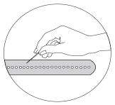
**WARNING:** A clogged venturi tube can cause a fire to occur beneath the Grill, due to a flashback of gas.
